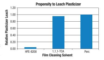
from Eastman Color Negative (ECN) and Eastman Color Intermediate (ECI) film. This data is for comparison purposes only. Results are shown below with the amount leached by perchloroethylene equal to 1.00.
